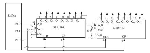
When serial port is working in MODE0, the serial data is input/output from RXD(P3.0) pin and serial clock is output from TXD(P3.1). Serial data is always starting transmission from the lowest bit.
