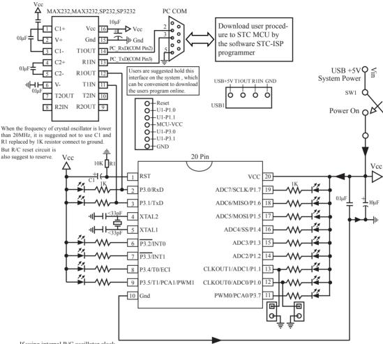
If using internal R/C oscillator clock (4MHz ~ 8MHz, manufacturing error), XTAL1 and XTAL2 pin should be floated.
