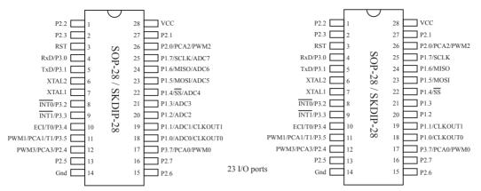
STC12C5620AD series (with A/D Converter), 28-Pin
