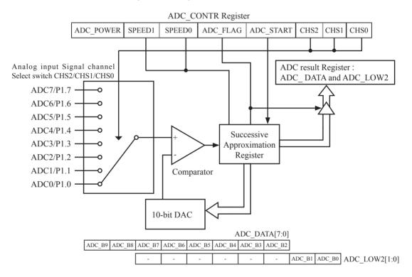
The ADC on STC12C5620AD is an 8-bit resolution, successive-approximation approach, medium-speed A/D converter.  $V_{REFP}/V_{REFM}$  is the positive/negative reference voltage input for internal voltage-scaling DAC use, the typical sink current on it is 600uA ~ 1mA. For STC12C5620AD, these two references are internally tied to VCC and GND separately.
