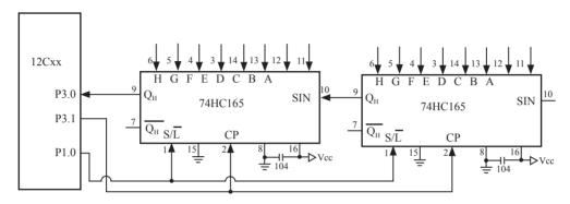
74HC165 is a 8-bit parallel input shift register, when S/L (Shift/Load) pin is falling to low level, the parallel port data is read into internal register, and now, if S/L is raising to high and ClockDisable pin (15 pin) is low level, then clock signal from CP pin is enable. At this time register data will be output from the Dh pin (9 pin) with the clock input.
