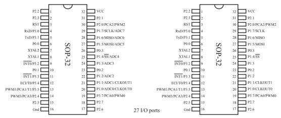
STC12C5620AD series (with A/D Converter), SOP-32
