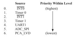
Note that the "priority within level" structure is only used to resolve simultaneous requests of the same priority level.
