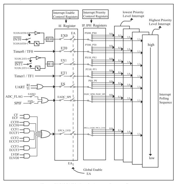
Figure STC12C5620AD series Interrupt Structure diagram
