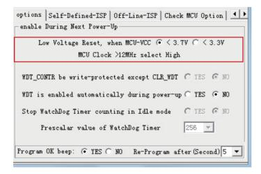
The detection voltage of 3V MCU of STC12LE5620AD series is optional between 2.4V and 2.0V as shown in following figure.
