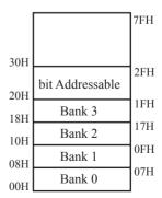
Lower 128 Bytes of internal SRAM
